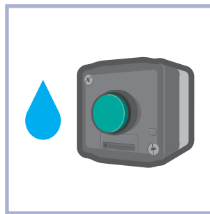
FIG. 2 Push function: the button stops and restarts water flow while assigned time continues to elapse.
