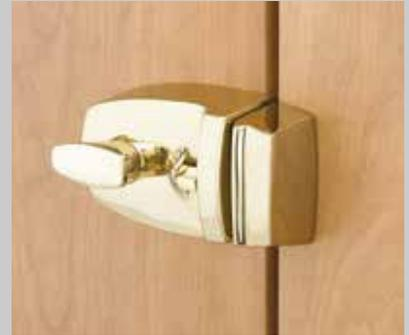
When selecting a replacement nightlatch, it is important to check that the backset (B) (ie. the measurement from the centre of the keyhole to the edge of the door) is the same as your existing lock. If you are fitting a lock to a new door, choose the longest backset that allows a comfortable fit.
