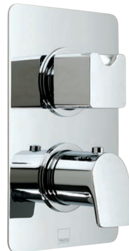
concealed 3 outlet, 2 handle thermostatic shower valve with integrated diverter 1.5 bar MP PHO-148C/3-C/P includes fittings for 1/2" and 3/4" pipework
