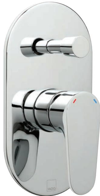
2 outlet concealed shower valve with diverter 0.2 bar LP (shower) 1.5 bar MP (bath) ASC-147A-C/P
