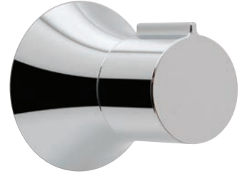
concealed 2 or 3 way diverter valve 0.2 bar LP (shower) 1.0 bar MP (bath) ALT-144-C/P note: to use as a 3 way diverter remove blanking plug
