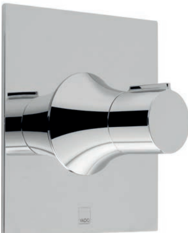
concealed thermostatic mixing valve 0.2 bar LP (shower) 1.0 bar MP (bath) ALT-163A-C/P note: this valve must be used in conjunction with a stop valve
