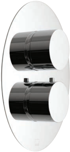
concealed thermostatic shower valve 0.2 bar LP SOH-148C-3/4-C/P includes fittings for 1/2" and 3/4" pipework
