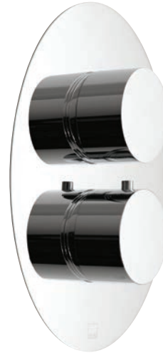
concealed 3 outlet, 2 handle thermostatic shower valve with integrated diverter 1.5 bar MP SOH-148C/3-C/P includes fittings for 1/2" and 3/4" pipework
